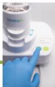
Press the Grind button (3 seconds) Then Sort (10 Seconds) Repeat until all particles are gone
